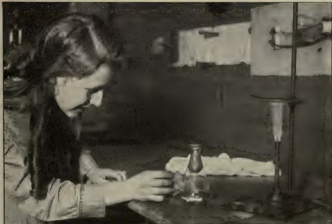
FIG. 53. As the steam condenses and leaves a vacuum, the air pressure forces the balloon into the flask.
